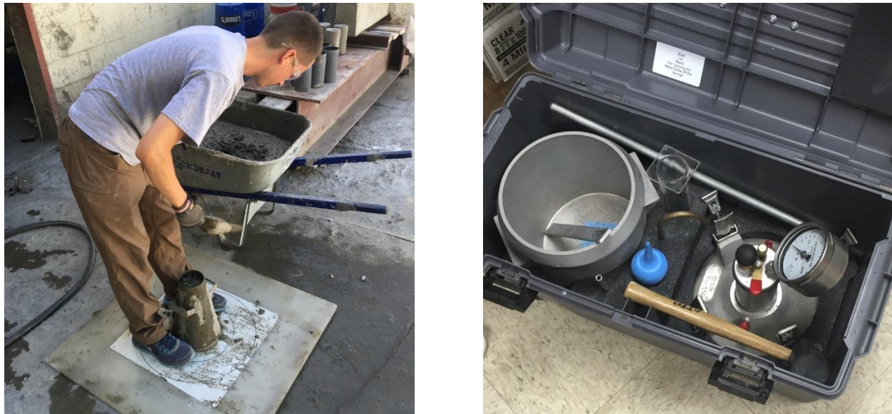
Figure 3.4 – Sump, Unit Weight, and Air Content Measurements
